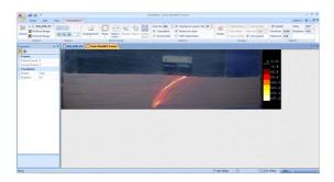
VSG software GUI (graphical user interface), in which the shear strain of sand grains are shown imposed on the main image.
